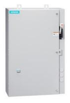
Non-reversing motor starter Size 0 Three phase full voltage Solid-state overload relay OLRelay amp range 3-12A 208VAC 60HZ coil Combination type 10Amp circuit breaker Encl NEMA type 4X 316 S-steel Water/dust tight noncorrosive Extra-wide enclosure
