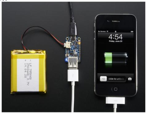
PowerBoost 500C is the perfect power supply for your portable project! With a built-in battery charger circuit, you'll be able to keep your project running even while recharging the battery! This little DC/DC boost converter module can be powered by any 3.7V Lilon/LiPoly battery, and convert the battery output to 5.2V DC for running your 5V projects.
