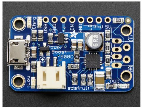
The PowerBoost 500C has at the heart a TPS61090 boost converter from TI (https://adafru.it/duQ). This boost converter chip has some really nice extras such as low battery detection, 2A internal switch, synchronous conversion, excellent efficiency, and 700KHz high-frequency operation. Check out these specs!
