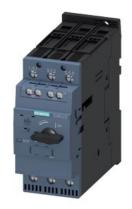
Circuit breaker size S2 for motor protection, Class 20 A-release 42...52 A N-release 741 A screw terminal Standard switching capacity with transverse auxiliary switches 1 NO+1 NC
