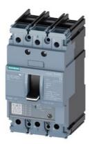
circuit breaker 3VA5 UL frame 125 3-pole, starter protection TM120M, AM, In=25A without overload protection short-circuit protection Ii=3...7 x In cable connection on both sides
