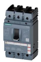
molded case switch 3VA5 UL frame 250 max. sh-circ breaking capacity 100kA @ 480 V 3-pole, line protection MCS110, In=150A without overload protection self-protection li=16 x In nut keeper kit on both sides
