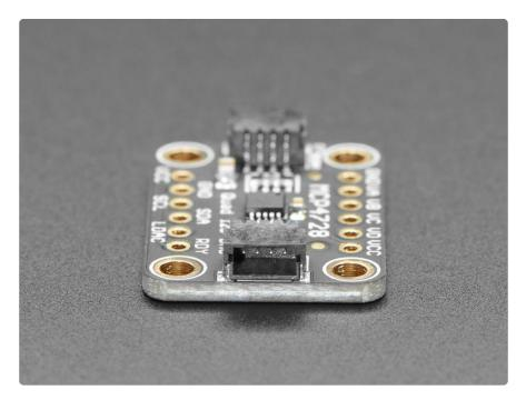
The breakout for the MCP4728 is populated with the required support circuitry to use it with your microcontroller of choice or Blinka-supported computer. The <u>SparkFun</u> <u>Qwiic</u> () compatible <u>STEMMA QT</u> () JST SH connectors ease the process of connecting the MCP4728 to your project and allows you to easily share an I2C bus with other STEMMA QT, Qwiic, Grove or other compatible sensors.
