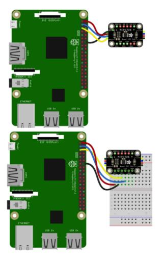
RPi 3.3V to MCP4728 VCC (red wire) RPi GND to MCP4728 GND (black wire) RPi SCL to MCP4728 SCL (yellow wire) RPi SDA to MCP4728 SDA (blue wire) Multimeter Positive Lead to MCP4728 VA, VB, VC, and VD in sequence Multimeter Negative Lead to GND
