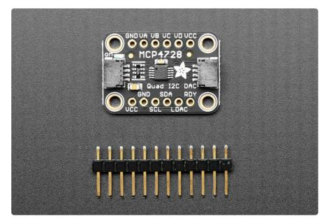
As of Aug 1, 2022 - we may make this board with the MCP4728 (default I2C address 0 x60) or MCP4728A4 (default address 0x64). To check your board's I2C address, use either the Arduino () or CircuitPython () I2C scanner programs.
