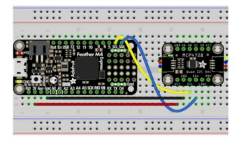
Feather 3.3V to MCP4728 VCC (red wire) Feather GND to MCP4728 GND (black wire)
