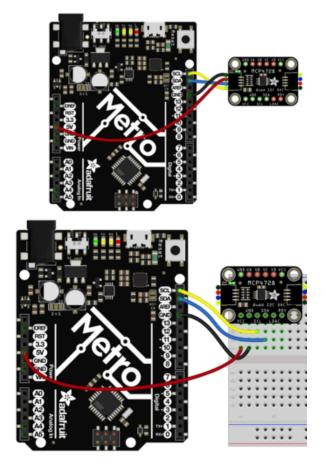
Arduino 5V to MCP4728 VCC (red wire) if you are running a 5V board Arduino (Uno, etc.). If your board is 3V, connect to that instead.
