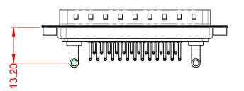
30A (CURRENT) POWER/CO-AX CONTACT RATING: (IF PRESENT) SIGNAL CONTACT CURRENT RATING: 5A PER CONTACT SIGNAL CONTACT RESISTANCE:  $10m\Omega$  MAX. **INSULATOR RESISTANCE:** 5000MΩ min.
