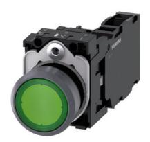
Illuminated pushbutton, 22 mm, round, plastic with metal front ring, green, pushbutton, flat, momentary contact type, with holder, 1 NO+1 NC, LED module with integrated LED 230 V AC, screw terminal, Z=20-unit packaging
