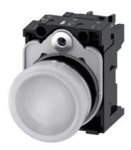
Indicator light, 22 mm, round, metal, shiny, white, lens, smooth, with holder, LED module with integrated LED 24 V AC/DC, screw terminal, with laser labeling, upper case and lower case, always upper case at beginning of line
