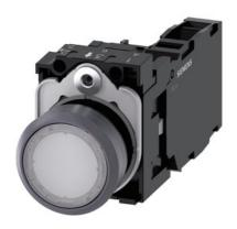
Illuminated pushbutton, 22 mm, round, plastic with metal front ring, white, pushbutton, flat, momentary contact type, with holder, 1 NO+1 NC, LED module with integrated LED 24 V AC/DC, screw terminal, with laser labeling, upper case and lower case, Always upper case at the beginning of the word
