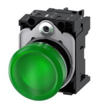
Indicator lights, 22 mm, round, metal, shiny, green, lens, smooth, with holder, LED module with integrated LED 24 V AC/DC, screw terminal, with laser labeling, inscription or symbol Customer-specific selection with SIRIUS ACT configurator (CIN)
