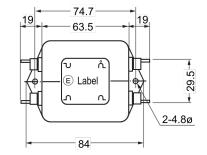
**General Information** Series GT Style Metal Box Description Noise Filters RoHS With Exemptions Qualifications UL, CSA, TUV Notes DC Available. Miscellaneous 35 K Self-Temperature Rise Max. Lead Fast On Terminal Type Faston
