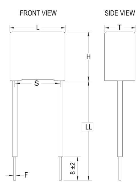
Click <u>here</u> for the 3D model. Dimensions L 26.5mm +0.3/-0.5mm
