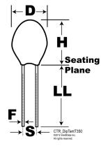
**General Information** Series T350 Dielectric MnO2 Tantalum Style Radial Description Radial, Solid Tantalum, Conformal, Dipped Features Low Leakage RoHS Yes Termination Tin AEC-Q200 No Notes Longest Lead Is Positive.
