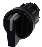
Illuminable selector switch, 22 mm, round, plastic, black, Selector switch short, 3 switch positions I-O-II, latching, actuating angle  $2x45^{\circ}$ , 10:30 /12 /13:30, Z=50-unit packaging
