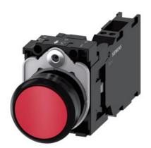
Pushbutton, 22 mm, round, plastic, red, pushbutton, flat, momentary contact type, with holder 1 NO+1 NC, spring-type terminal, with laser labeling, upper case and lower case, always upper case at the beginning of the word
