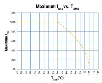
$T_{\text{AMB}}$  is the maximum ambient temperature surrounding the capacitor or hottest contact point (e.g. tracks), whichever is higher, in the worst operation conditions in °C.
