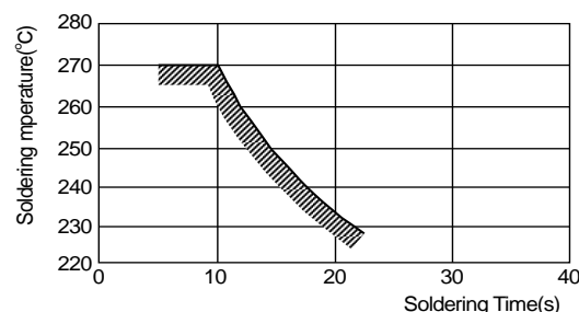
[Allowable Flow Soldering Temperature and Time]
