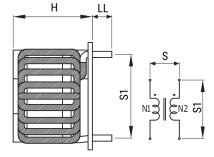
General InformationSeriesSC-JHStyleThrough-HoleRoHSYesNotesLead Spacing (S/S1) Are For Reference Only.MiscellaneousTemperature Rise Maximum: 85 K.CoreMn-Zn Ferrite
