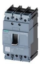
circuit breaker 3VA5 UL frame 125 breaking capacity class S 25kA @ 480 V 3-pole, line protection TM210, FTFM, In=100A overload protection Ir=100A fixed short-circuit protection Ii=10 x In UL489 SB (naval), 50 deg. cel. cable connection on both sides
