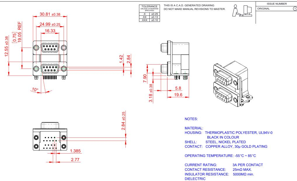
WITHSTANDING VOLTAGE: 1000V AC rms
