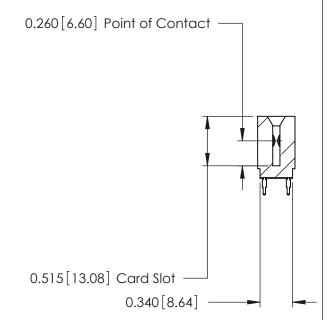
ACAD REFERENCE NO. 746-ENG MASTER 746 Series Ultra-Mate Card Edge Connector - Press Fit DRAWN: J.LEE DATE: AUG 20/09 Part Number: 746-052-520-201 CHECKED: DATE: **EDAC INC** SCALE: SHEET 1 OF 1 THESE DRAWINGS AND SPECIFICATIONS ARE THE PROPERTY OF EDAC INC.,AND TORONTO, ONTARIO SHALL NOT BE REPRODUCED, OR COPIED DRAWING NUMBER CANADA OR USED AS THE BASIS FOR THE 746-ENG MASTER MANUFACTURE OR SALE OF APPARATUS YOUR CONNECTION TO QUALITY & SERVICE WITHOUT WRITTEN PERMISSION.
