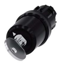
key-operated switch Siemens, 22 mm, round, plastic, lock number SSG10, with 2 keys, 2 switch positions O-I, latching, actuating angle  $90^\circ, 10:30h/13:30h,$  key removal O Z=50-unit packaging
