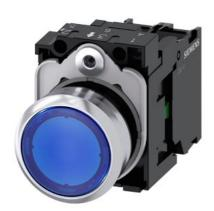
Illuminated pushbutton, 22 mm, round, Metal, shiny, blue, pushbutton, flat, momentary contact type, with holder, 1NO, LED module with integrated LED 230 V AC, screw terminal, with laser labeling, symbol number according to, ISO 7000 or IEC 60417
