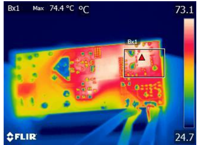
Figure 25 – Ambient = 24.7 °C. SR FET, Q3 = 74.4 °C.
