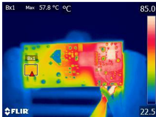
Figure 39 – Ambient = 22.5 °C. Bridge Diode, BR1 = 57.8 °C.
