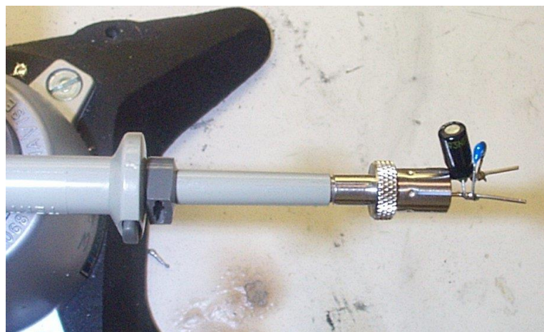
Figure 76 – Oscilloscope Probe with Probe Master ( www.probemaster.com ) 4987A BNC Adapter. (Modified with wires for ripple measurement, and two parallel decoupling capacitors added)
