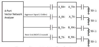
Figure 6. Channel-Isolation Test Configuration
