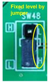
Jumper indicated in the left figure is adopted on this evaluation board to set operation of the TB67S141FTG.
