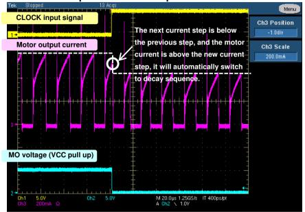
When the current step is shifted to the next step: if the motor current is above the PWM threshold, it will then go onto the decay sequence. If the motor current is below the next current step, it will continue on to the constant current PWM.
