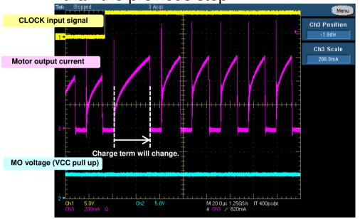
When the current threshold (current step) is shifted to the next threshold (step), the 'Charge' time may change, but the 'Decay (=off time)' time will not. (The off time depends on the OSCM resistance.)
