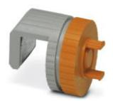
The optional holding device ensures the Rogowski coil is securely seated on busbars with a thickness of 10 ... 15 mm. During installation, the coil housing is pushed onto the flange of the holding device and snaps in automatically.
