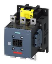
Contactor, AC-1, 400 A/690 V/40  $^{\circ}$ C, S10, 3-pole, 96-127 V AC/DC, F-PLC-IN with varistor, 2 NO+2 NC, permanently mounted, Connection rail/ screw terminal
