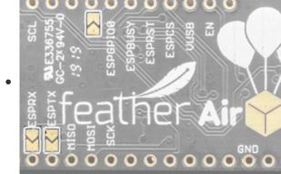
Make sure to solder each of these pads together. You will not be able to upload firmware to your ESP32 if they are not connected.
