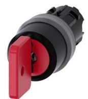
Key-operated switch O.M.R, 22 mm, round, plastic with metal front ring, lock number 73037, red, with 2 keys, 3 switch positions I>O<II, momentary contact type, actuating angle 2x45°, 10:30h/12h/13:30h, key removal O, with laser labeling, upper case and lower case, always upper case at beginning of line
