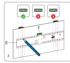
Using the marking template (E) provided, mark four holes for drilling on the centerline of the stud.
