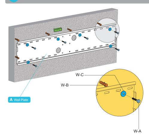
3 Place concrete anchors (W-B) in each hole. Tap each anchor flush with the wall using a hammer. Using a socket wrench, mount the wall plate (A) and fasten them with the provided lag bolts (W-A) and D8 washers (W-C).
