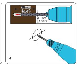
Using a power drill and 1/4" drill bit, drill pilot holes of 1/4" (6 mm) diameter and at least 3.5" (90 mm) depth.
