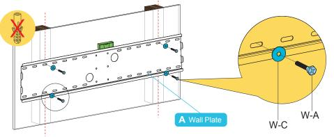
5 Mount the wall plate (A) and tighten it with the provided lag bolts (W-A) and D8 washers (W-C) using a socket wrench.
