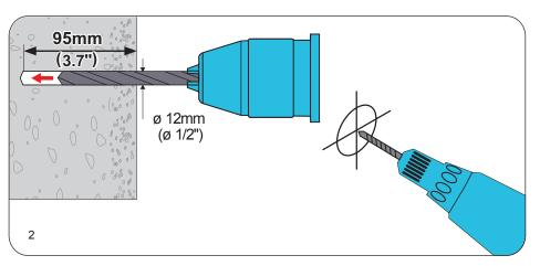
Using a power drill and a 1/2" masonry drill bit, drill mounting holes of 1/2" (12 mm) diameter and 3.7" (95 mm) depth at the marked locations in the previous step.
