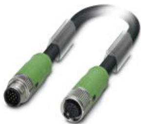
Sensor/actuator cable, 17-pos., PUR/PVC, RAL 9005 (black), shielded, straight M12 SPEEDCON male plug (A-coded) to straight M12 SPEEDCON female plug, cable length: 5 m
