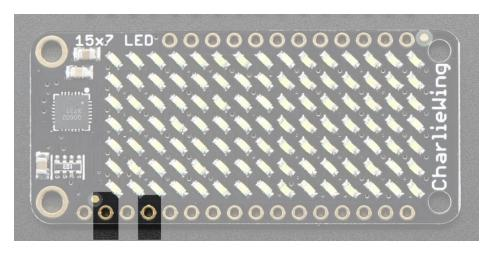
The LED matrix uses only the **3V** (second from left) and **GND** (fourth from left) pins for power and logic. Current draw depends on how many LEDs are lit but you can approximate it as about 40mA for most uses.
