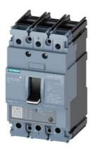
circuit breaker 3VA5 UL frame 125 3-pole, starter protection TM120M, AM, In=30A without overload protection short-circuit protection li=5...12 x In cable connection on both sides
