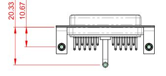
POWER/CO-AX CONTACT RATING: 20A (CURRENT) (IF PRESENT) SIGNAL CONTACT CURRENT RATING: 5A PER CONTACT SIGNAL CONTACT RESISTANCE:  $10m\Omega$  MAX.
