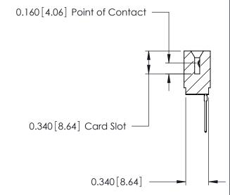
ACAD REFERENCE NO. 746 Series Ultra-Mate Card Edge Connector - Press Fit DRAWN: J.LEE Part Number: 746-032-545-501 CHECKED: SCALE: **EDAC INC** THESE DRAWINGS AND SPECIFICATIONS ARE THE PROPERTY OF EDAC INC.,AND TORONTO, ONTARIO SHALL NOT BE REPRODUCED, OR COPIED DRAWING NUMBER CANADA OR USED AS THE BASIS FOR THE 746-ENG MASTER MANUFACTURE OR SALE OF APPARATUS
