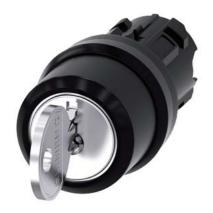
RONIS key-operated switch, 22 mm, round, plastic, lock number 455, with 2 keys, 3 switch positions I-O-II, latching, actuating angle 2x45°, 10:30h/12h/13:30h, Key removal I+O+II, with laser labeling, upper case and lower case, always upper case at the beginning of the word
