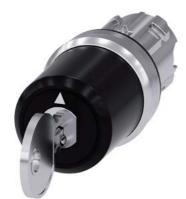
key-operated switch Siemens, 22 mm, round, metal, shiny, lock no. STGH10, with 2 keys, 3 switch positions I-O<II, left latching, momentary contact type on the right, actuating angle 2x45°, 10:30h/12h/13:30h, key removal O+I, with laser labeling, upper case and lower case, always upper case at beginning of line
