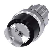
RONIS key-operated switch, 22 mm, round, metal, shiny, lock number 455, with 2 keys, 2 switch positions O-I, latching, actuating angle 90°, 10:30h/13:30h, key removal O, with laser labeling, upper case and lower case, always upper case at beginning of line
