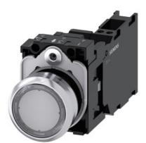
Illuminated pushbutton, 22 mm, round, metal, shiny, clear, pushbutton, flat, momentary contact type, with holder, 1 NO+1 NC, LED module with integrated LED 110 V AC, spring-type terminal, with laser labeling, upper case and lower case, always upper case at beginning of line
