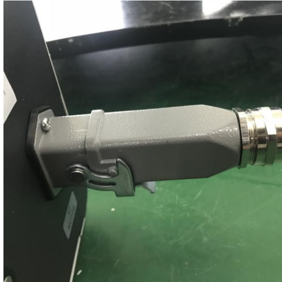
Figure 4.3 Connect controller and robot by heavy-duty cables
