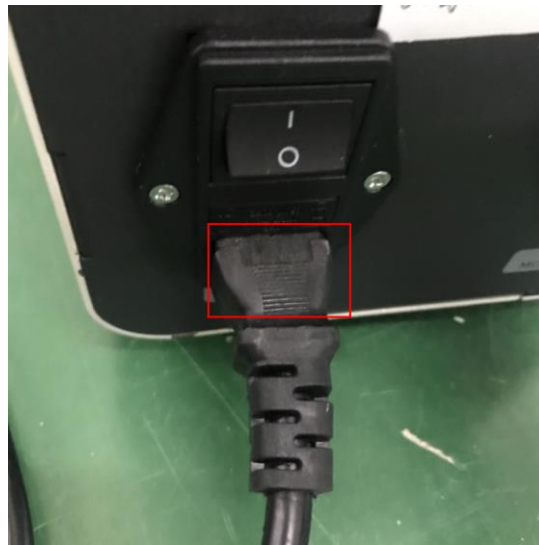
Figure 4.6 Connecting to Power Supply
