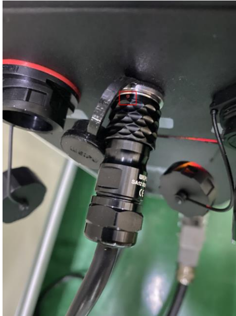
Figure 4.4 Connecting emergency stop switch
