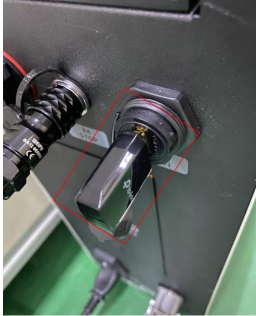
Figure 4.5 Connecting WiFi module
