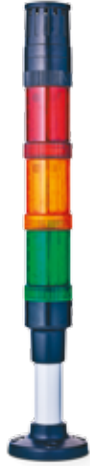
Order number: ECO40-Q81 Colours: red/orange/green Function: LED steady beacon, buzzer steady or pulsing tone Nominal voltage: 230 V AC Type of mounting: Tube mounting (100 mm tube length)
