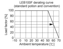
Calculating A<sub>1</sub>, A<sub>2</sub>, A<sub>3</sub> A<sub>1</sub>=I<sub>O1</sub>/I<sub>1</sub>×100=0.2/5×100=4  $A_2=I_{02}/I_2\times 100 = 2/4\times 100 = 50$  $A_3=(V_1\times Io_1+V_2\times Io_2)/(TOTAL OUTPUT WATTAGE)\times 100$ =(5×0.2+24×2)/100×100=49
