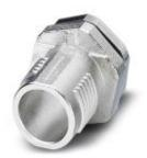
M12 SPEEDCON housing screw connection for M12 male inserts, with O-ring, for all SPEEDCON-capable THR and wave soldering contact carriers
