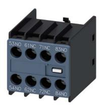
Auxiliary switch on the front, 2 NO + 2 NC Current path 1 NO, 1 NC, 1 NC, 1 NO for contactor relays Size S00 screw terminal 53/54, 61/62, 71/72, 81/82 Physically coded; only with contactor relays 3RH2140\* and 3RH2440\* can be combined (according to EN 50011)
