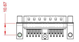
POWER/CO-AX CONTACT RATING:75Ω (IMPEDANCE)(IF PRESENT)SIGNAL CONTACT CURRENT RATING:5A PER CONTACTSIGNAL CONTACT RESISTANCE:10mΩ MAX.
