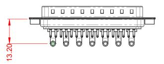
20A (CURRENT) POWER/CO-AX CONTACT RATING: (IF PRESENT) SIGNAL CONTACT CURRENT RATING: 5A PER CONTACT SIGNAL CONTACT RESISTANCE:  $10m\Omega$  MAX. **INSULATOR RESISTANCE:** 5000MΩ min. DIELECTRIC
