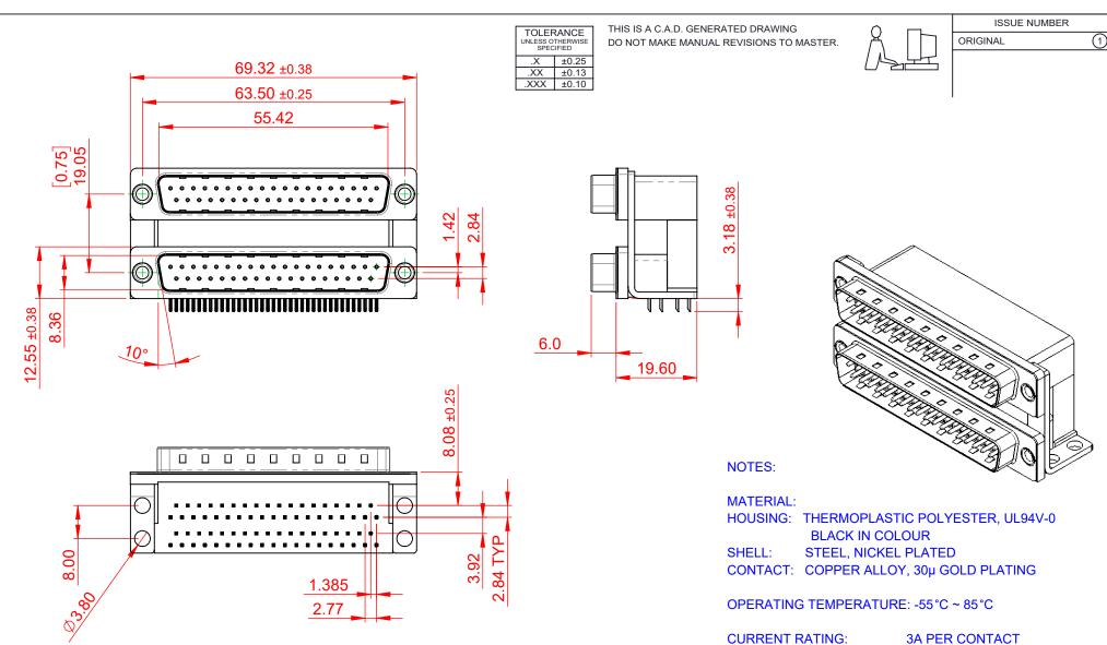
CURRENT RATING:3A PER CONTACONTACT RESISTANCE: $25m\Omega$  MAX.INSULATOR RESISTANCE: $5000M\Omega$  min.DIELECTRICWITHSTANDING VOLTAGE:1000V AC rms
