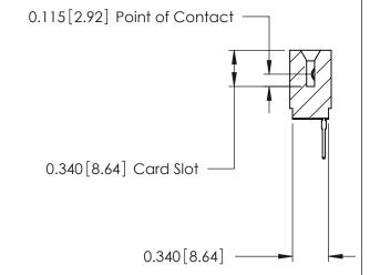
ACAD REFERENCE NO. 746 Series Ultra-Mate Card Edge Connector - Press Fit DRAWN: Part Number: 746-034-527-501 CHECKED: **EDAC INC** THESE DRAWINGS AND SPECIFICATIONS ARE THE PROPERTY OF EDAC INC.,AND TORONTO, ONTARIO SHALL NOT BE REPRODUCED, OR COPIED CANADA OR USED AS THE BASIS FOR THE MANUFACTURE OR SALE OF APPARATUS
